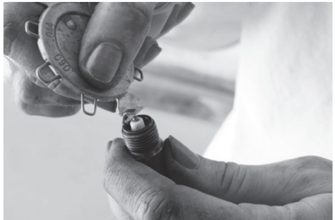
Figure 5-19. Adjust Spark Plug Gap
